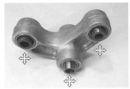
• Draw out the cushion lever bearings with the special tool.
