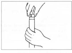
• Install the oil seal stopper ring ⑤ and the dust seal ⑥.
