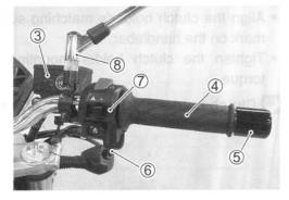
Apply SUZUKI SUPER GREASE to the throttle cable and the cable drum.
