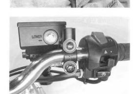
Remove the brake lever ② and brake light switch ③.
