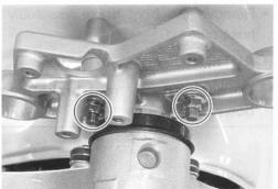
Remove the steering stem upper bracket by removing the steering stem head nut.
