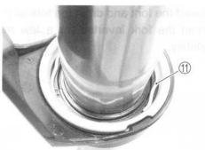
· Pull the inner tube out of the outer tube with light impact.
