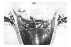
Remove the cowling inner cover by removing the screws ①
