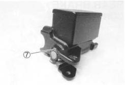
Install the brake lever and brake light switch.
