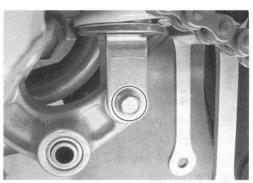
• Remove the rear shock absorber 1.
