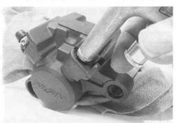
Remove the dust seal ⑤ and piston seal ⑥.
