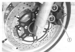
• Slightly loosen the front axle by using the special tool.
