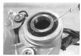
Remove the steering stem lower bearing ⑤.
