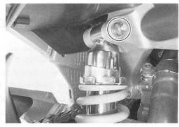
• Remove the rear shock absorber lower mounting bolt.
