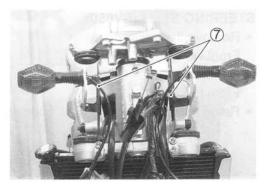
• Loosen the handlebar holder nuts lightly.
