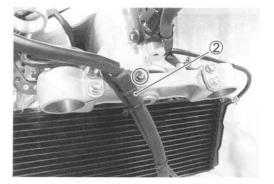
Remove the steering stem nuts with the special tools.
