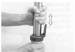
Hold the front fork vertically and adjust the fork oil level with the special tool.
