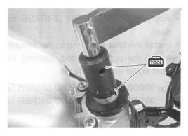
Install the handlebar holders and then tighten the handlebar holder nuts to the specified torque. (SV650)
