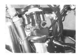
Remove the front brake assembly by removing the brake hose guide ②.
