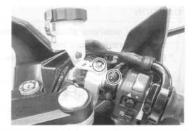
Remove the reservoir from the master cylinder.
