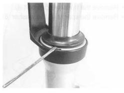
Remove the oil seal stopper ring ①.
