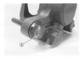
Place a rag over the piston to prevent it from popping out and then force out the piston using compressed air.
