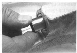
Remove the swingarm pivot bearing and spacer with the special tools.
