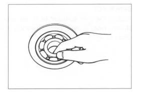
Remove the sprocket mounting drum bearing and wheel bearings by using the special tool.
