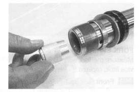
. Insert the inner tube into the outer tube and fit the oil seal and dust seal with the special tool.
