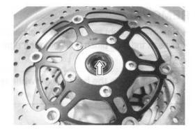
· Remove the dust seal by using the oil seal remover.
