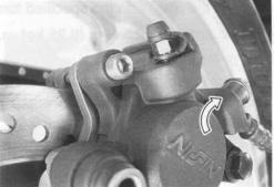
• Assemble the new brake pad 4, insulator 5 and shim 6.
