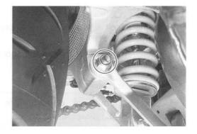
• Remove the rear shock absorber upper mounting bolt.
