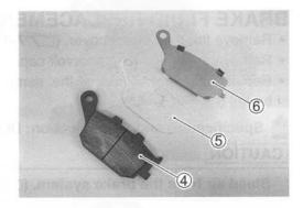
· Install the new brake pads and pad mounting pin.
