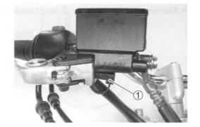
Place a rag underneath the union bolt on the master cylinder to catch any spilt brake fluid. Remove the brake hose union bolt and disconnect the brake hose.
