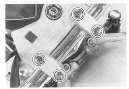
Remove the handlebars by removing the handlebar clamp bolts.
