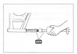
• Remove the cushion rod bearings by using the special tool.
