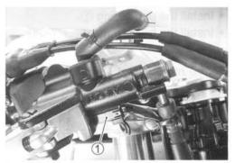
Place a rag underneath the union bolt on the master cylinder to catch any spilt brake fluid. Remove the brake hose union bolt and disconnect the brake hose.
