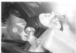
· Loosen the front fork lower clamp bolts.
