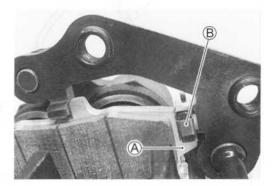
Install the inner pad so that the inner pad will be seated on the hatched part ©.
