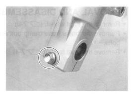
• Remove the cylinder bolt ®.
