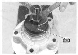
First install the right wheel bearing, then install the left wheel bearing and spacer using the special tool.
