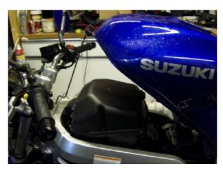
3: Undo the tank retaining bolts... Lift the tank & prop up with the tank prop (surprisingly!!) 4: Run the engine until at it's normal operating temperature (most are around 85 - 90 deg)
