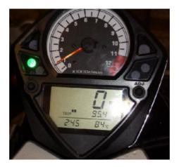
6: If (as above) the idle is too low, locate the idle adjust screw – on the left hand side of the bike in one of the triangle shapes in the chassis and adjust. Turn clockwise to raise the idle speed and anti-clockwise to lower it... Go in small movements and 'blip' the throttle after each adjustment and allow it to settle before trusting what the rev counter says!
